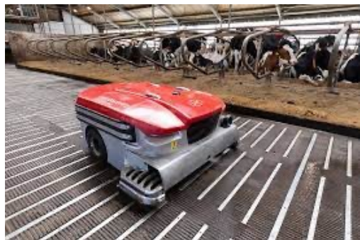
Lely Sphere with feces collector
