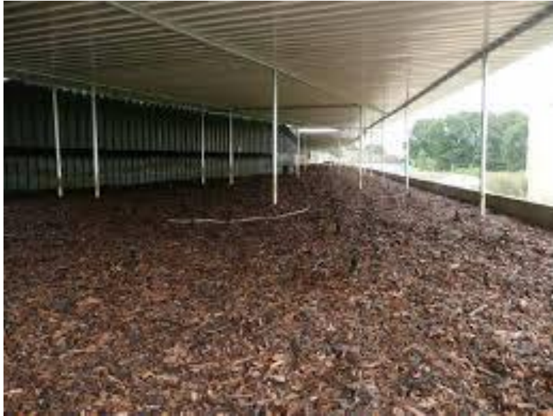
Biobed with wood chips
