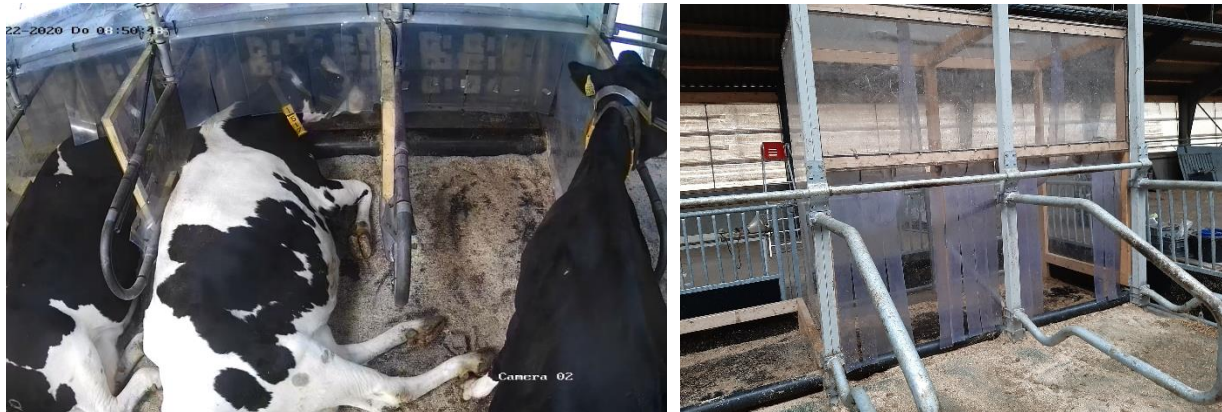
Figure 2. Measuring methane concentrations in methane box at cow end of cubicle (Left Netherlands, right Denmark)
