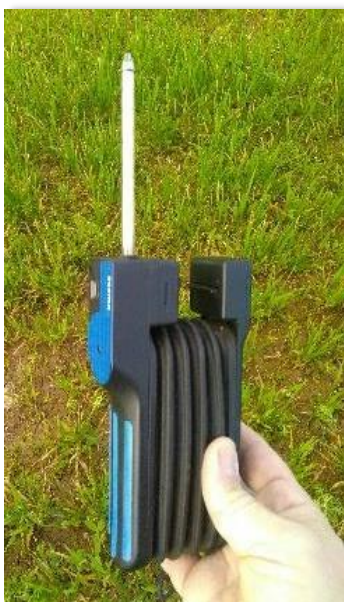
Figure 9 : Colorimetric tubes used for ammonia emission measurements and the associated pump
