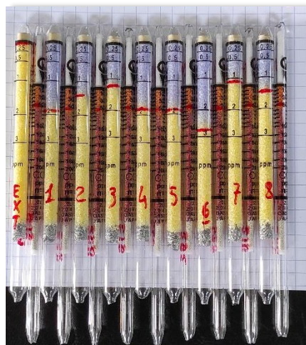
Figure 9 : Colorimetric tubes used for ammonia emission measurements and the associated pump
