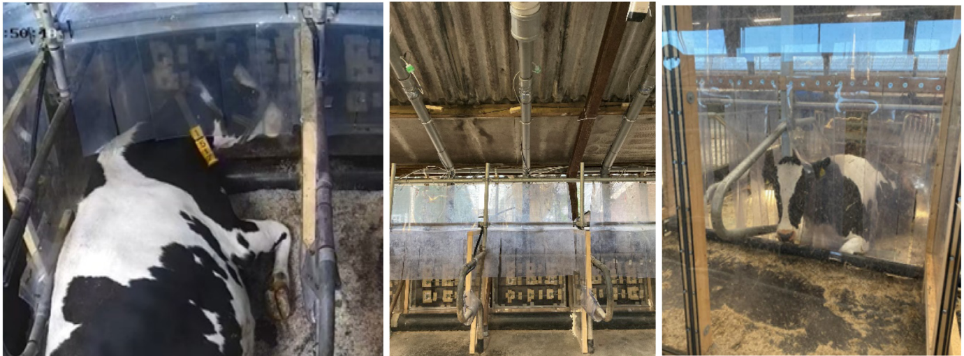
Figure 2. Cows in box with hood for capturing methane (experimental setups). Left and center: Levraut (2024); right: M. Myllerup (SEGES, Aarhus, Denmark, personal communication).
