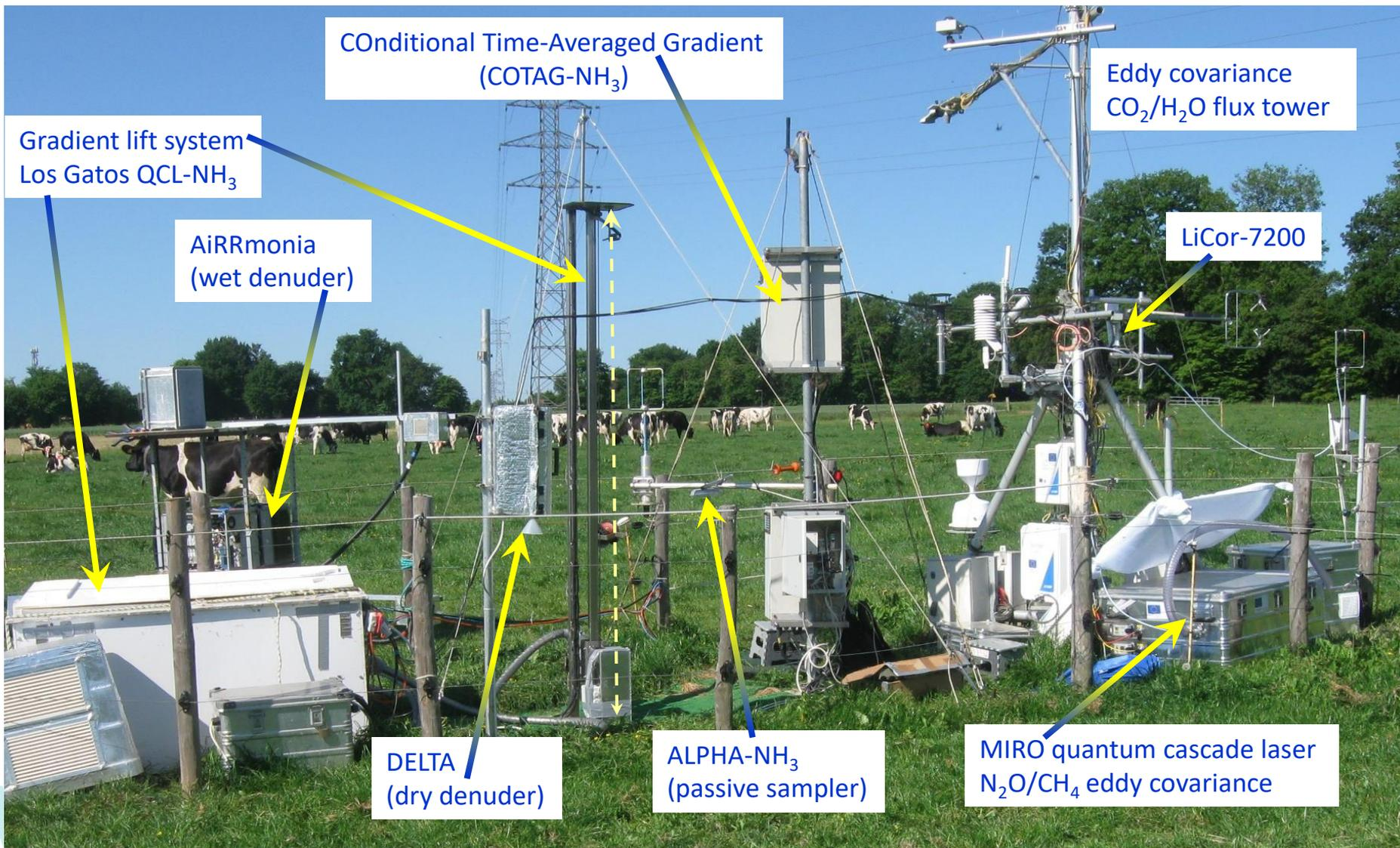
➤ Grazing-related NH<sub>3</sub> emissions: aerodynamic gradient method using Los Gatos quantum cascade laser (QCL) & lift system
